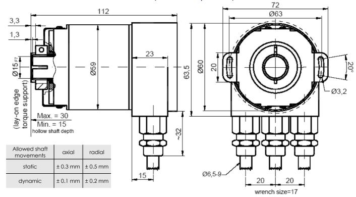
Shaft diameter can be reduced to 12mm, 10mm or 8mm by reduction ring (by inserting them into the hollow shaft)
